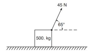
The horizontal component of the force acting on the crate is
